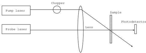
**Figure 10:** Schematic of an optical switching setup
