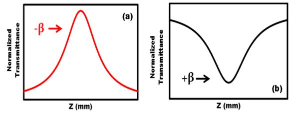
**Figure 3:** Open aperture z-scan traces (a) saturable absorption and (b) reverse saturable absorption curves
