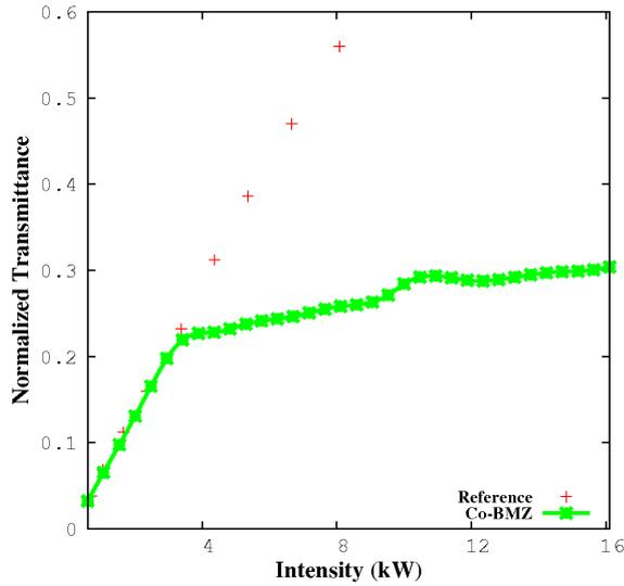
**Figure 8:** *Optical limiting of Co-BMZ thinfilms*
