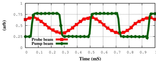
**Figure 11:** Demonstration of optical inverter switch in Mn-BMZ film
